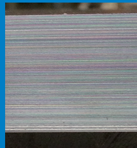
P-PE0804T：加工表面良好 Favorable Machined Surface
